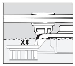
The water level is correct when dimensions "X" is at least 1/8" (4 mm).
